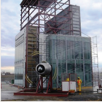
Figure 9: Exterior mock-up test (AAMA 501) - UL – CLEB laboratory
