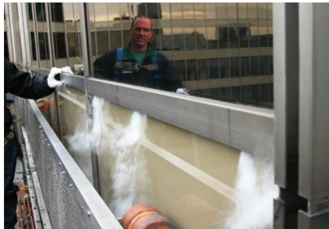
Figure 27: Excessive smoke exfiltration visible on exterior side of curtain wall test specimen
