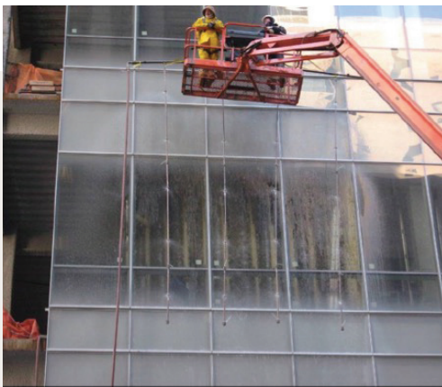
Figure 17: Identification of representative area for field testing (metal and glass curtain wall)
