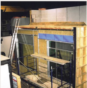
Figure 10: Interior mock-up test (CAN/CSA-A440) - Air-Ins laboratory
