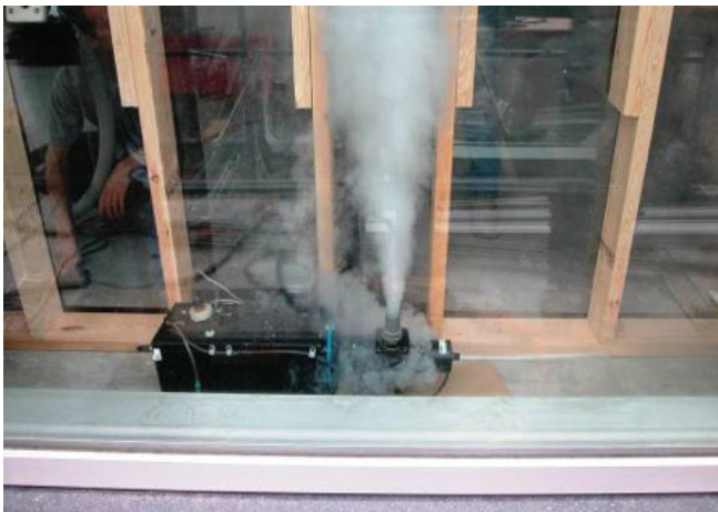
Figure 26: Portable smoke generator used to fill test chamber with white smoke
