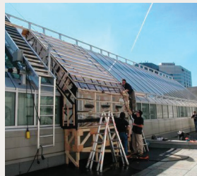
Figure 22: Exterior test chamber used to test a skylight section
