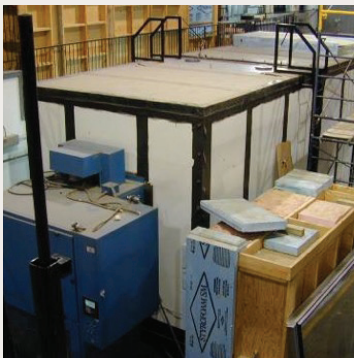
Figure 11: Environmental test chamber at the UL – CLEB laboratory
