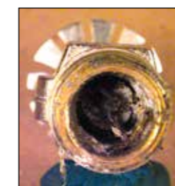
Figure 2: Photograph illustrating the level of deposits commonly found in sprinkler inlets.
