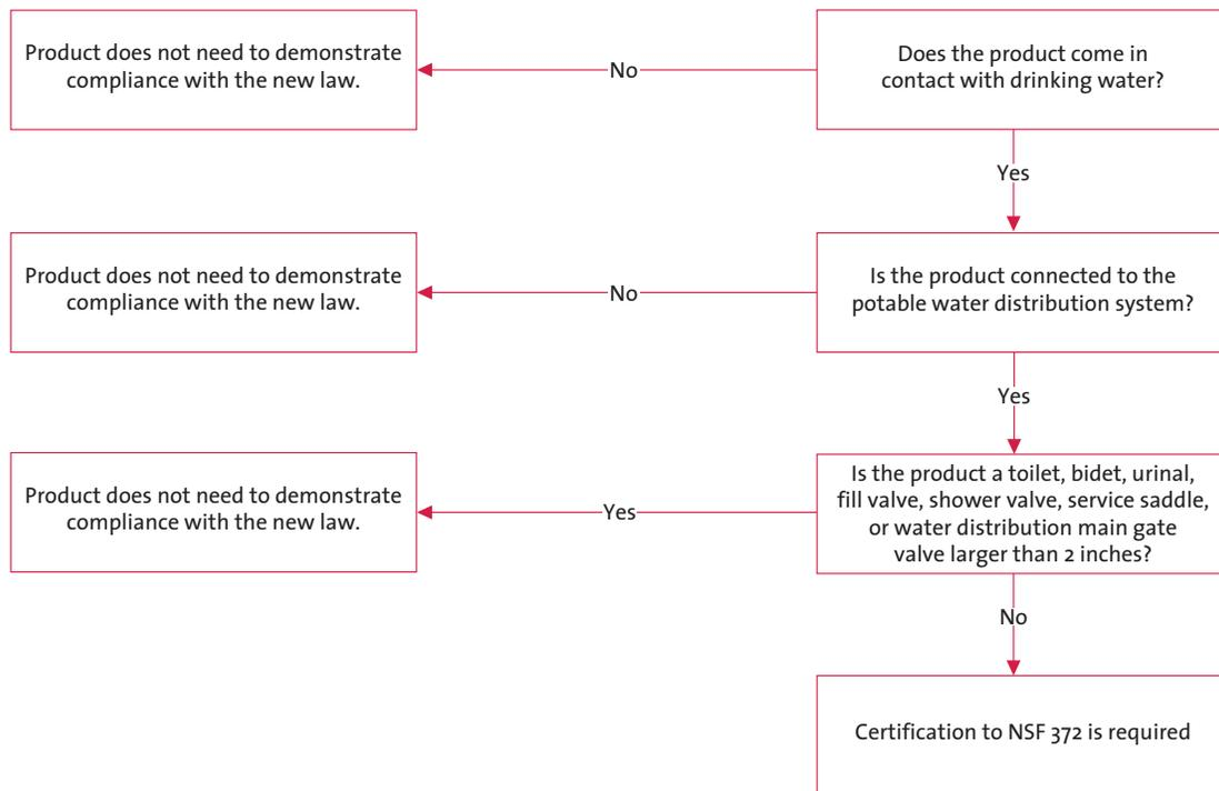
These requirements cover the evaluation of wetted surfaces of products, components, and materials that convey or dispense water that is intended for human consumption by drinking or cooking for lead (Pb) content.
