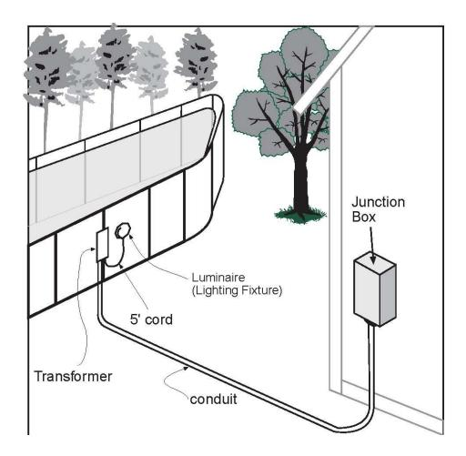
Fig. 2 - Underwater Luminaire for aboveground non-storable swimming pool.
